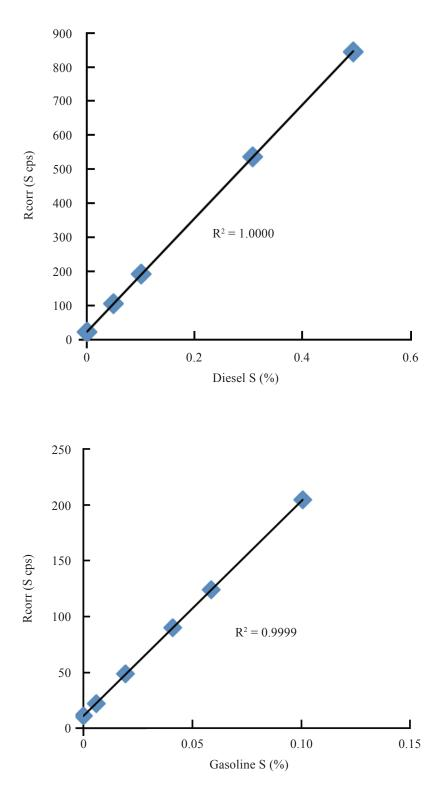
Figure 1. Diesel and gasoline calibration line.
