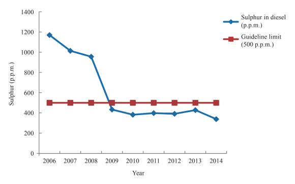
Figure 3. Median diesel sulphur concentration over the period 2006 to 2014.
