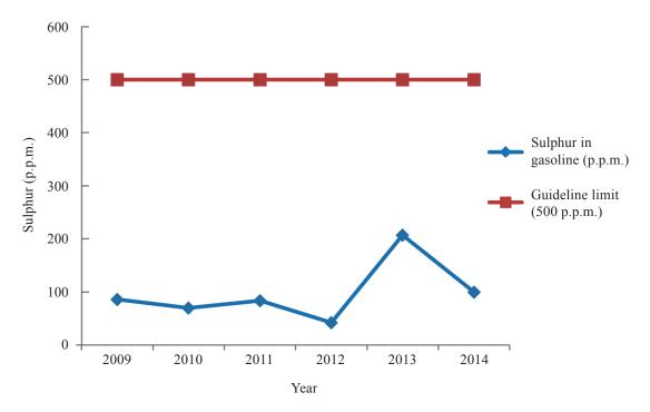
Figure 4. Median gasoline sulphur concentration over the period 2009 to 2014.
